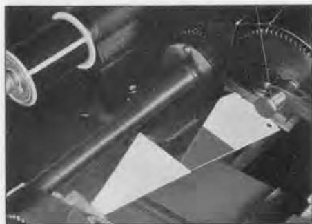
Figure 8. Close-up of the double sawtooth during winding, showing how the mandrel is clamped in the lathe.
