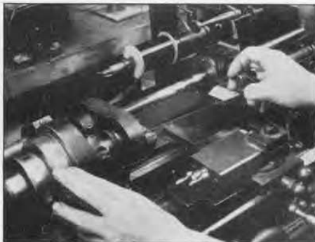
Figure 9. Hand winding, as shown here, is often used on steeply sloping mandrels.
