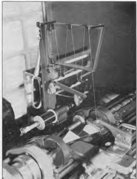
Figure 5. View of double-sawtooth card being wound. Note the arrangement of pulleys and springs to take up variations in tension as the card is rotated.
