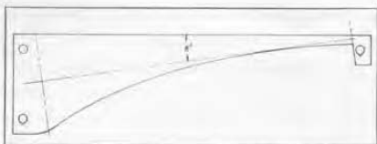
Figure 10. Mandrel widths are laid out perpendicular to the winding axis as shown here by the center line.
